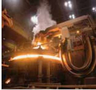
Aqualoy shafting starts with careful selection of raw materials combined and melted in an electric arc furnace.
