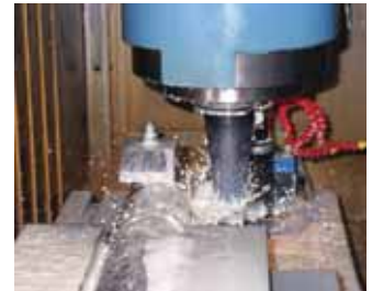
CNC milling of keyway, a value-added service to our distributors.
